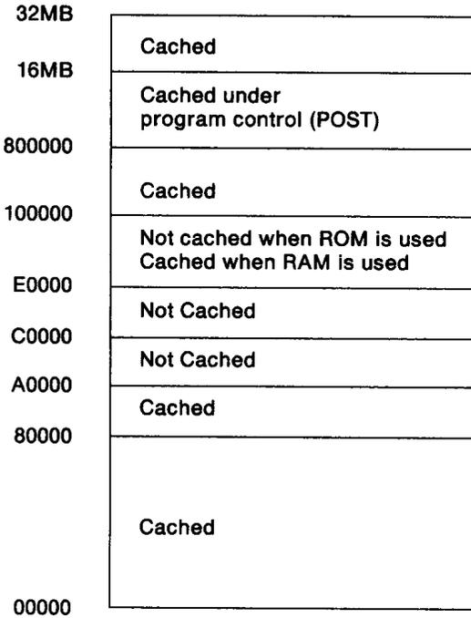
*Figure 3-6. Mapping of the First 32MB Segment*
